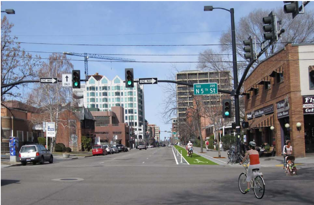
Figure 4: Protected Bike Lane with Parking Removed (Idaho at 5 th )
