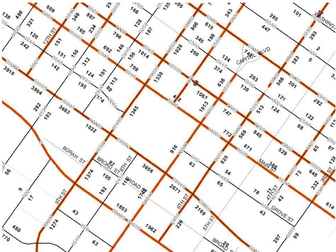
Peak-hour traffic counts (in black) suggest the number of lanes that are needed to handle Demand.
