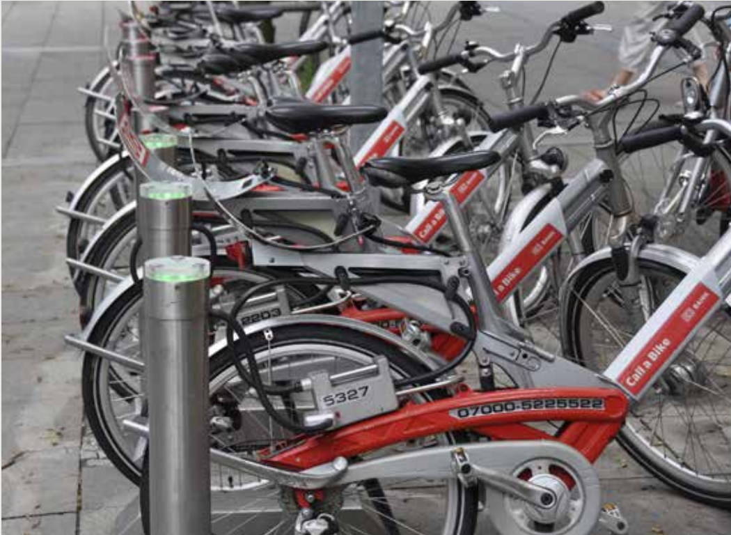
LEFT Stuttgart, Germany, implemented a bike-share system that includes electric bikes with chargers at stations and GPS location devices.
