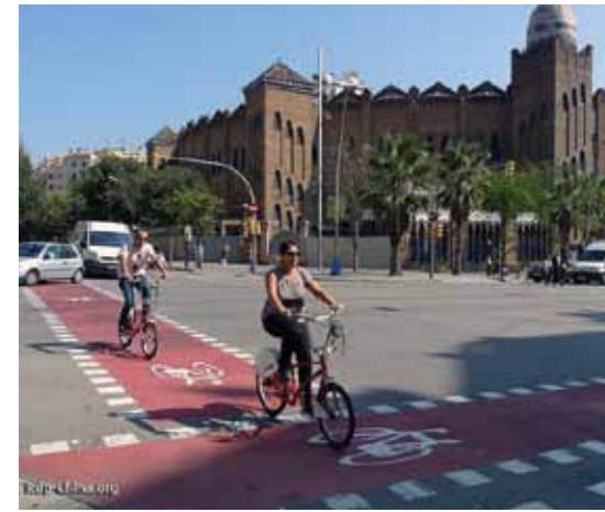
Striping the bike lane through the intersection is a clear indicator that bike traffic is expected and drivers should watch out especially when turning. Barcelona, Spain.
