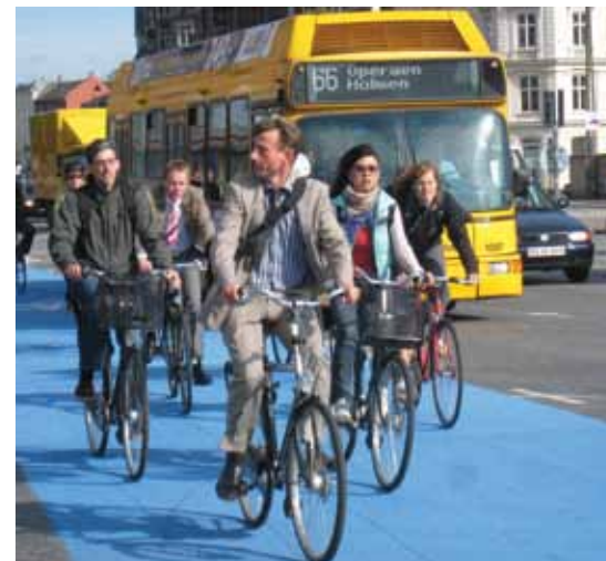
Blue dedicated lanes at intersections increase awareness and safety.
