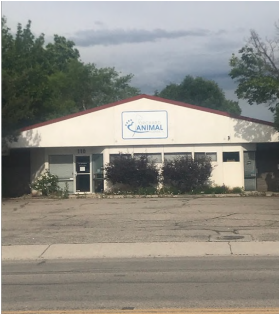
Lack of access management on North Orchard Street. Managed access points, such as right-turn driveways, encourages drivers to slow down to enter the parking lot, and makes the road safer and more comfortable for pedestrians.
