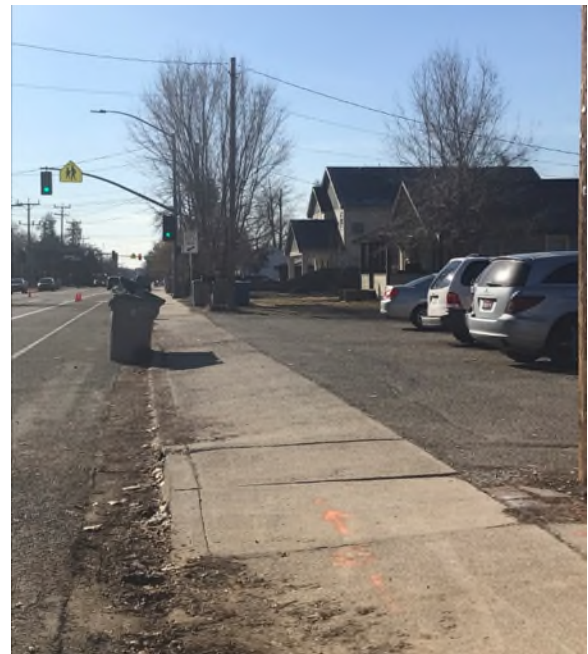
South Latah Street. This photo shows access to and parking for an eight-bedroom single-family home outside of the photo to the right. The wide driveways and pull-in/pull-out parking configuration creates a hazard to pedestrians and bicyclists and the lack of permeable surface increases the burden on stormwater infrastructure.
