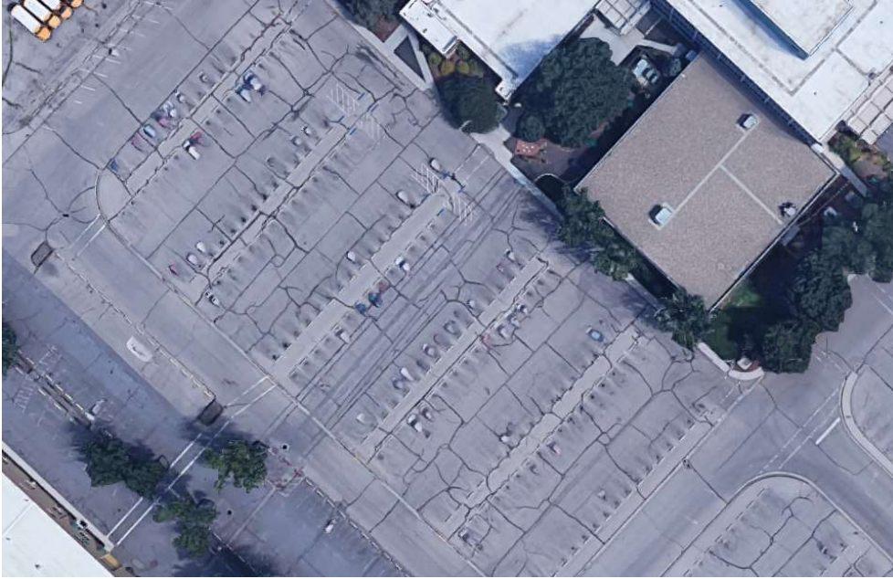
ITD parking lot deterioration
