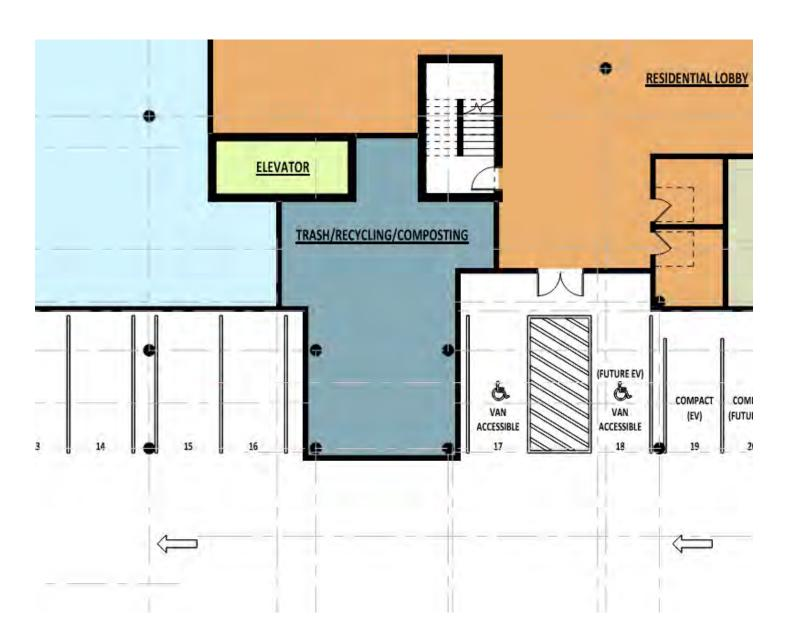
See SD plan snip below for proposed EV (1 stall) and future EV (7 stalls) locations. EV stall counts and locations may shift, but will meet LEED Silver thresholds for quantity and proximity to building access.
