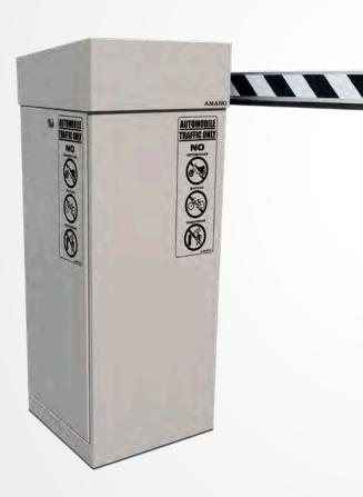
The AMI-1200 Series Universal Barrier Gate is designed to control vehicles in both attended and unattended parking traffic lanes by means of a straight or folding aluminum gate arm. The on-board microprocessor provides flexible lane logic, control and functionality and supports three switch-selectable modes of operation to meet the needs of customer applications.
