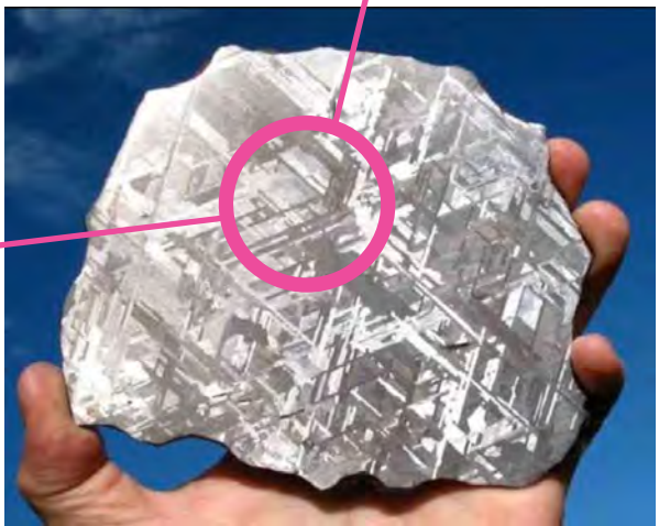
IRON - CRYSTAL LATTICE "WIDMANSTATTEN PATTERN" (VID-man-shtay-tin)
